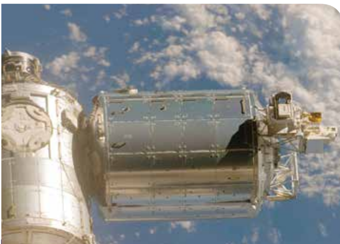
The European Technology Exposure Facility attached to the Columbus module of the International Space Station during orbital flight.
